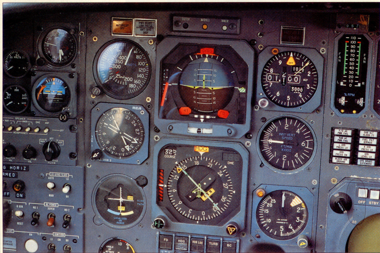
Big and businesslike, the CE-500's bull's-eye flight director (below) was state of the art in the early 1970s. Easy to read and fly, some high-timers yearn for its return.
